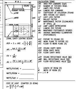
U = UNIT COST OF LIGHT FOR A LAMP (DOLLARS/10<sup>6</sup> Im x h)
